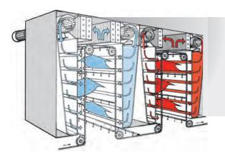
An even flow in the heating and cooling zones for different drying processes
