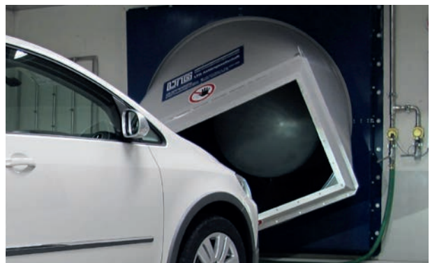
Fahrtwind-Simulator type VAF 2240 - outlet nozzle rotatable by 360°
